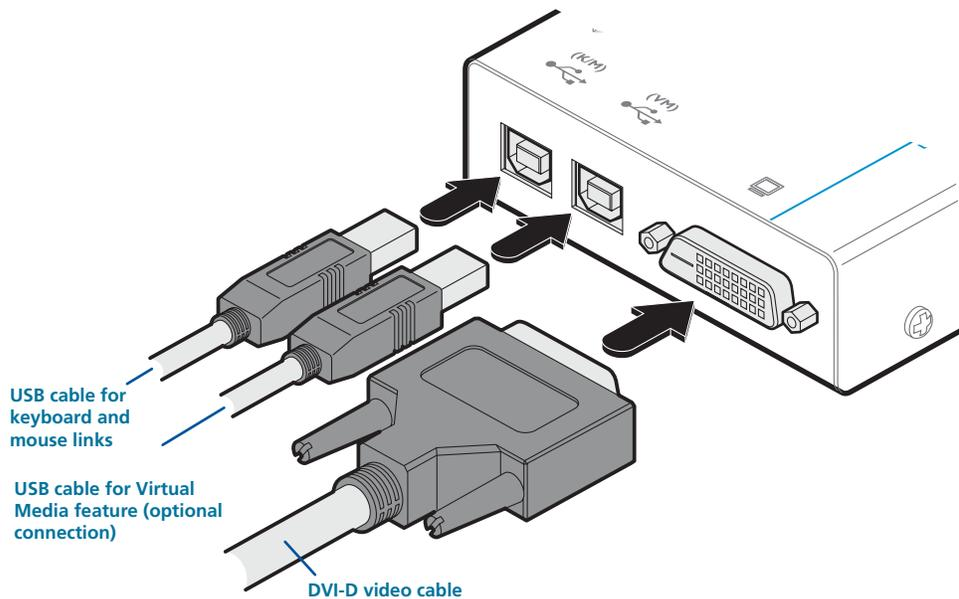
Figure 3-3. Connecting the video and USB cables
