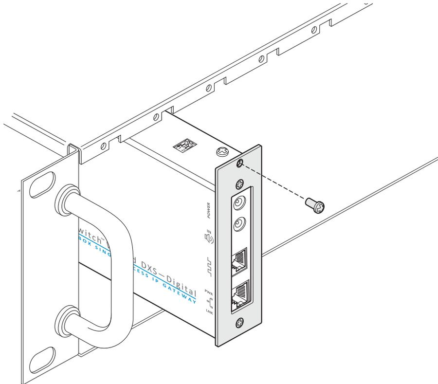
Figure 3-2. Fixing the module into the rack
