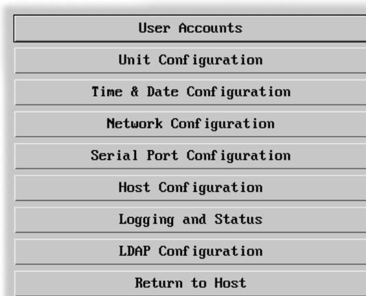
Use the various options (particularly the 'Unit Configuration' and 'Network Configuration' options) to arrange the Wizard DXS - Digital to suit your requirements.
