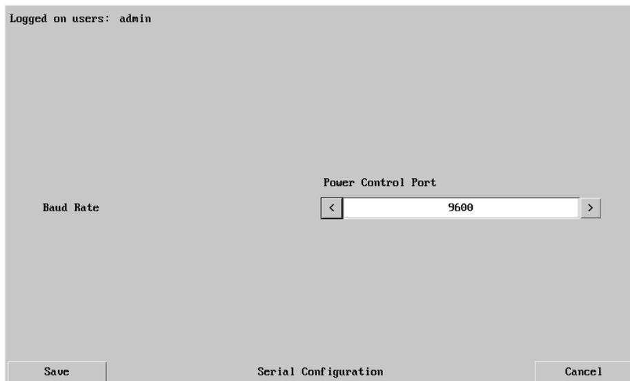
The screenshot shows a web-based configuration interface. At the top left, it says "Logged on users: admin". The main area is titled "Serial Configuration". On the left, there is a label "Baud Rate". In the center, there is a "Power Control Port" dropdown menu with "Power Control Port" selected. Below the dropdown is a numeric input field with a value of "9600" and left and right arrow buttons. At the bottom, there are three buttons: "Save", "Cancel", and "Serial Configuration".
