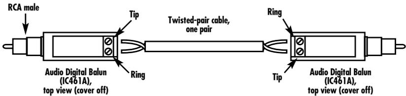
**Figure 3-1. Straight-through polarity.**
