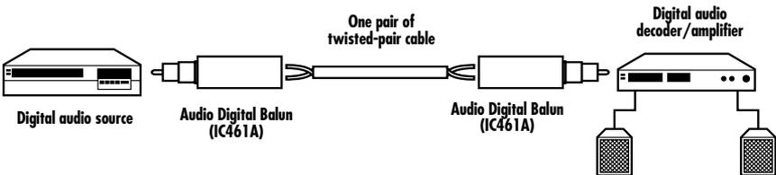
**Figure 3-2. Typical installation.**
