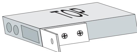
c. Save the unused tabs in a safe place or secure them to the chassis' unused slots.
