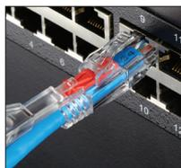
Gently pull back the Locking Pin. Lift up the Tool to release it from the Locking Pin.
