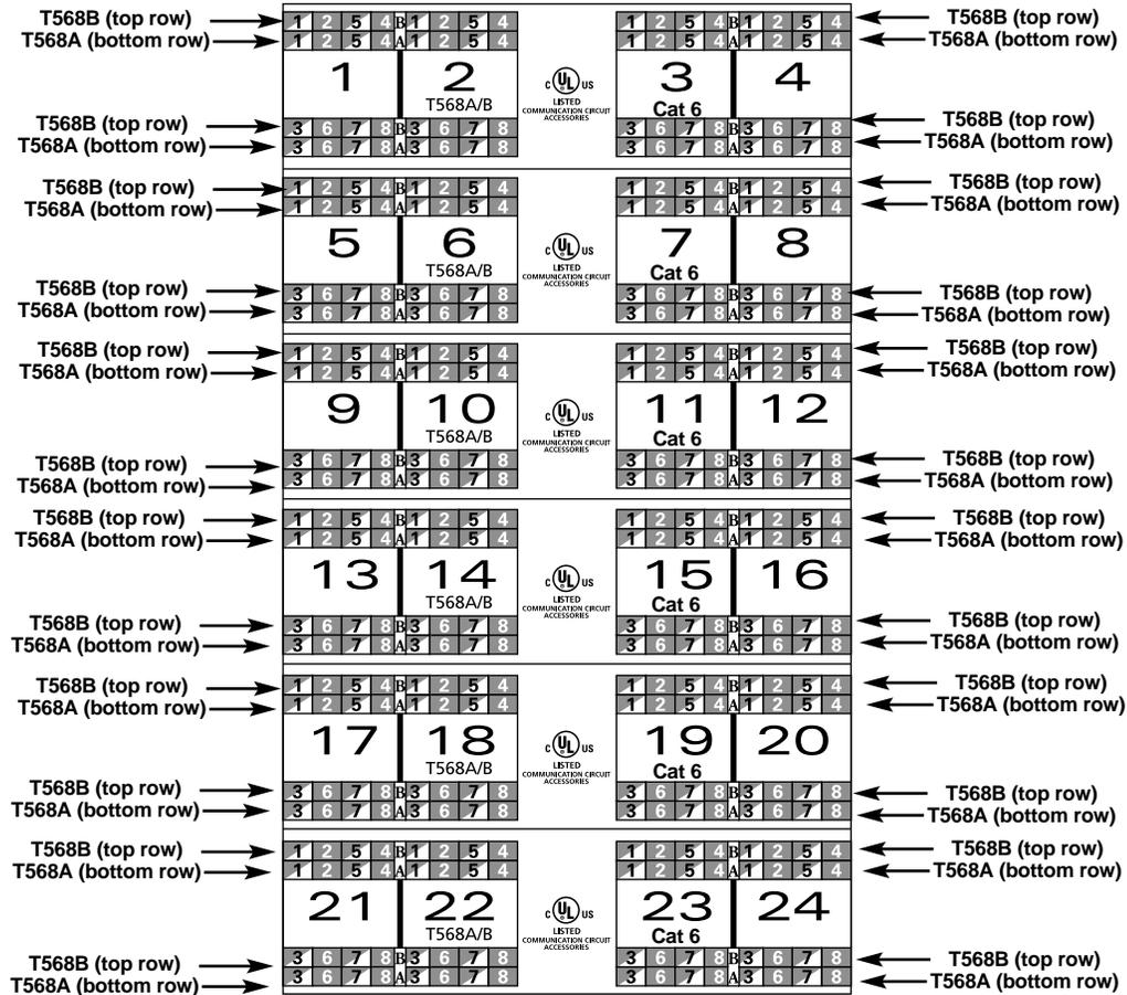
Figure 5. 24-port patch panel's T568B and T568A wiring sticker labels.
